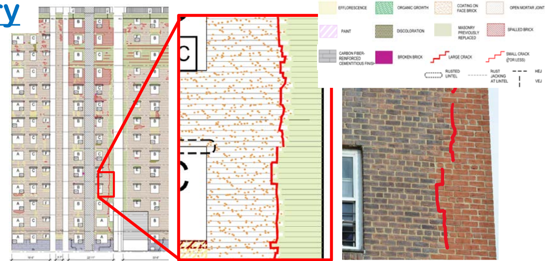
Building 5 (1141 FDR Drive) Damage Mapping
